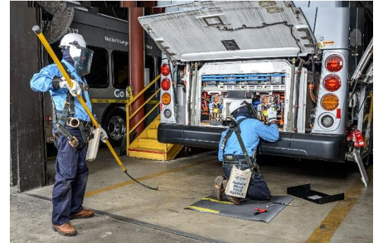
Figure 1 Technicians performing maintenance on a BEB
