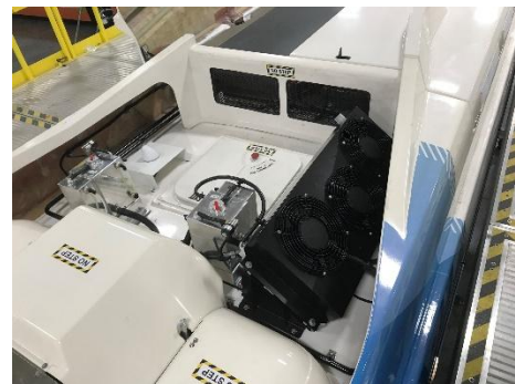
Figure 33 BEB expansion tanks
