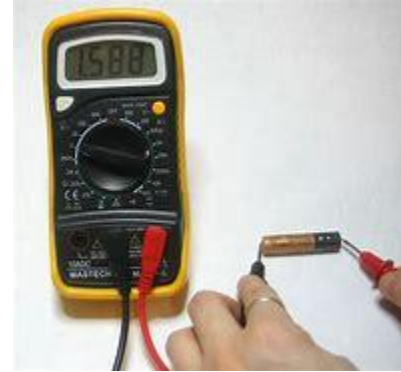
Figure 83 Digital multimeter in use
