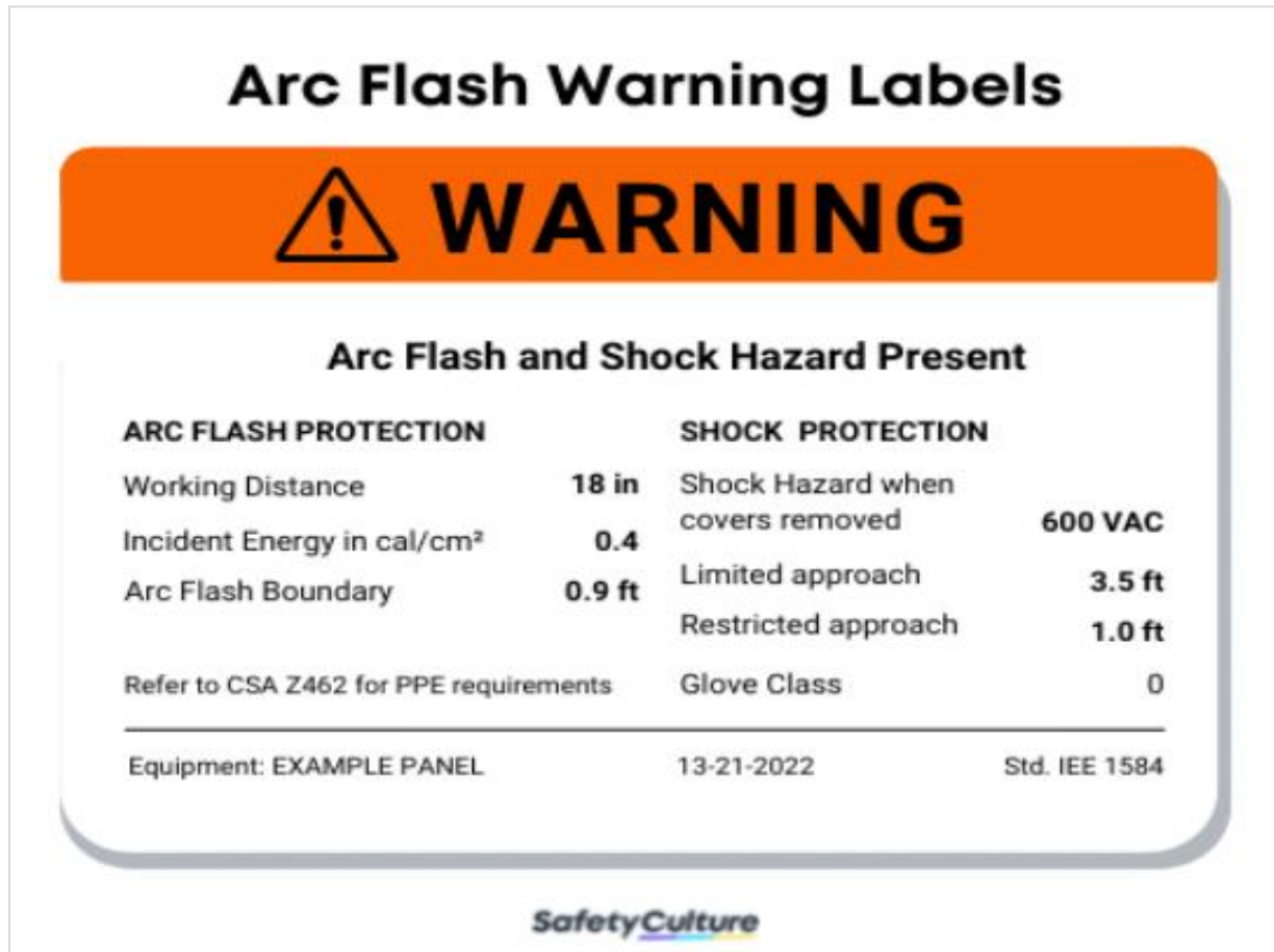
Figure 65 Example Arc Flash Warning Label
