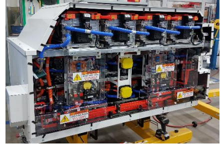
Figure 54 Low Voltage Distribution Box
