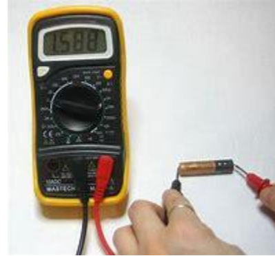
Figure 83 Digital multimeter in use
