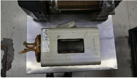
Figure 20 Water cooled rotary vane with an AC motor diagram and drive motor – courtesy AC Transit
