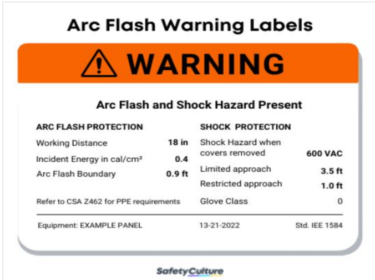
Figure 65 Example Arc Flash Warning Label
